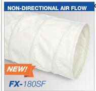
Construction: High strength sewn single-ply PVC vinyl coated polyester fabric hose reinforced with a spring steel wire helix and external PVC wearstrip
