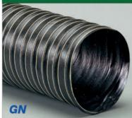
Construction: Double-ply neoprene coated fiberglass fabric hose reinforced with a spring steel wire helix & external filament fiberglass cord.
