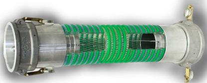
Internally grounding the hose between the two fittings eliminates concerns if the embedded grounding wire has become detached/broken within the hose or from the fittings. This safety feature is available on all of our grounded fuel delivery hoses.
