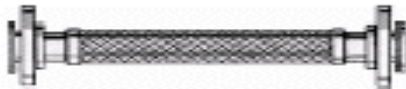
316 Stainless Steel Corrugated Metal Hose with a 304 Stainless Braid and *Flange Retainers With Carbon Steel 150# Flanges Each End (Gaskets Optional)
